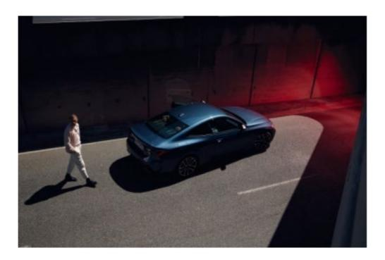
With this upgrade, the system also brakes when reversing for pedestrians whose current movement indicates that a collision with the rear of the vehicle may be imminent.
