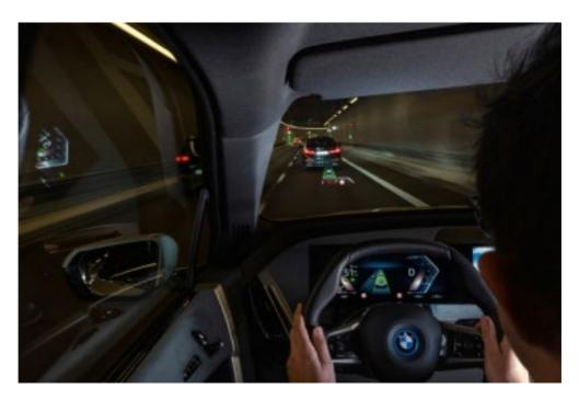
You can now display the familiar Assisted Driving View functions (e.g. Steering Assistant) as a visualization in the Instrument Cluster and Head-up Display.
